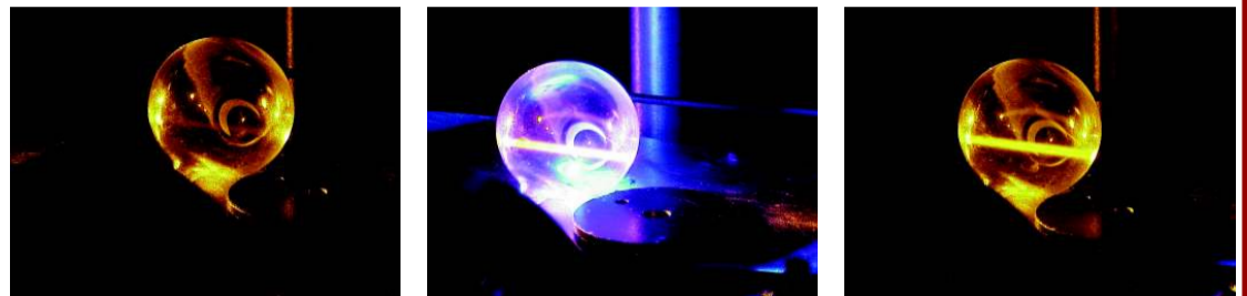
Fig. 2: Images of the PDMS coated cell at RT. Left: 200 mW dye laser; center: 200 mW dye laser, LIAD system on; right: 200 mW dye laser, LIAD system on, seen through optical filter.
